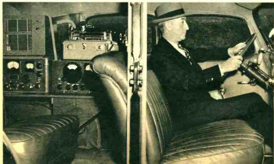
SPECIALY-EQUIPPED CARS ACT AS MECHANICAL BLOODHOUNDS, FOLLOWING SIGNALS OF AN ILLEGAL TRANSMITTER TO THEIR SOURCE
